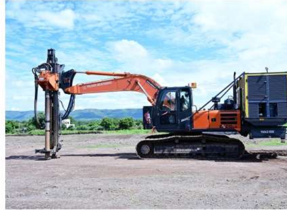
SOLAR DTH PILING MACHINE
